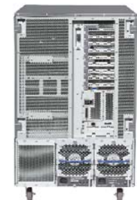
Back, I/O connectors and power supplies
