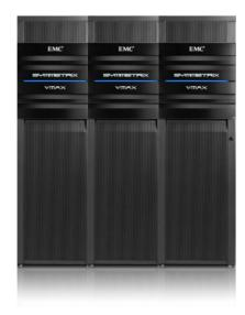
VMAX 40K high-density configurations support up to 3,200 drives, consuming 33 percent less space, 35 percent less weight, and 27 percent less power compared with 3.5-inch drives.
