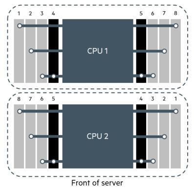
**BL460c Gen10 DIMM Channels and Numbering**
