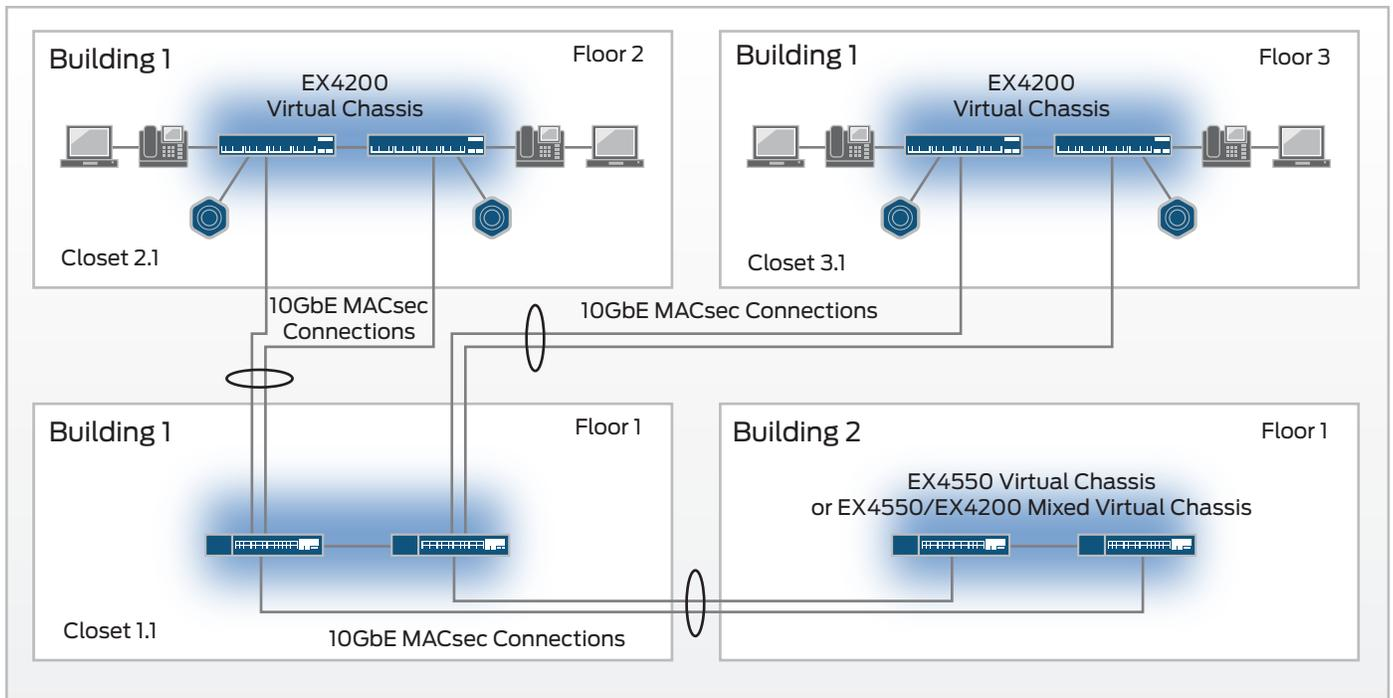
Figure 2: MACsec deployment with EX4200 and EX4550 switches.
