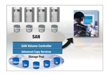
IBM System Storage SAN Volume Controller is designed to virtually consolidate capacity from different storage systems, help provide common copy functions and enable data movement without server disruption, while supporting management of diverse storage from a single point.
