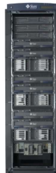
Three Sun Fire 3800 servers and three Sun StorEdge D240 Media Trays in a Sun Fire cabinet
